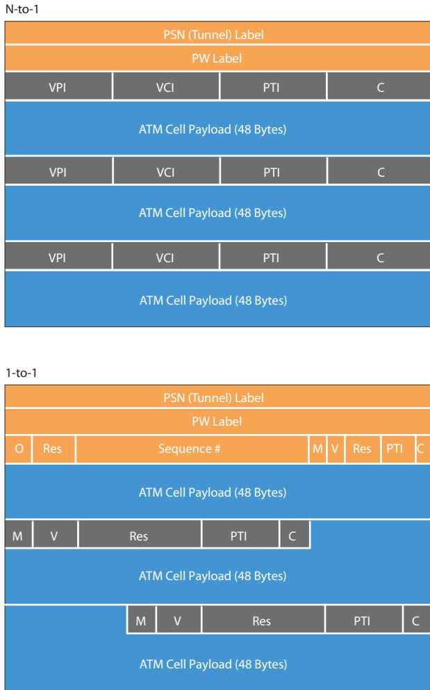
Figure 11. ATM cell concatenation in MPLS pseudowires
