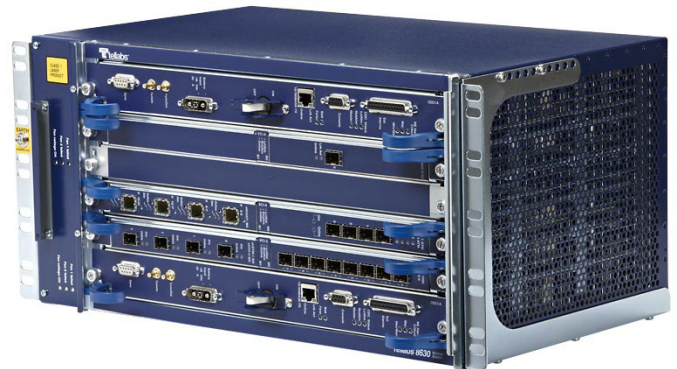
The Tellabs 8630 is an IP/MPLS-based switch/router integrating a complete set of carrier-class functions
